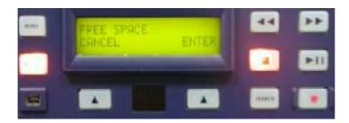
To determine the amount of FREE SPACE available for you to store additional DV files on your **DV Bank**, press the **MENU** key until the word FREE appears in the top left corner of the LCD, then press the Soft Key below the word ENTER. The total amount of free space available will appear in the top right corner of the LCD and is shown in hours, minutes, seconds and frame number. Pressing the Soft Key under CANCEL will take you back to the previously selected FILE screen.
